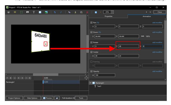
• The "Rotate X" Control will rotate an Object about its Centre Point in 3 Dimensions Vertically:
