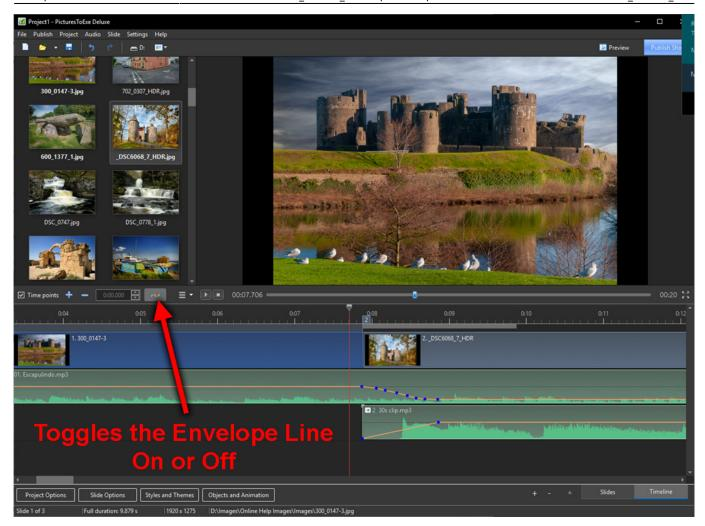
• The Colors of the Envelope Line, Waveform, Keypoint and Shading can be selected in the Timeline Tab of Settings / Preferences.
